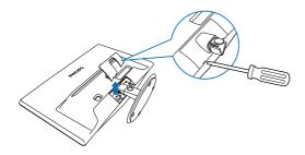
2. Remove the 4 screws and then remove the base from the monitor.
