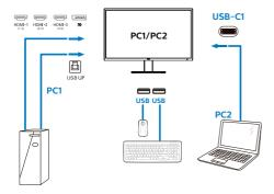
3. Enter to OSD menu. Go to KVM layer and select "Auto", "USB-C1" or "USB up" to switch the control of peripherals from one device to another. Simply repeat this step for switching the control system using one set of peripheral.
