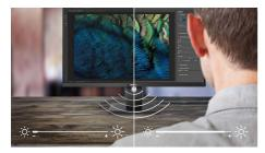
PowerSensor is a built-in 'people sensor' that transmits and receives harmless infrared signals to determine if user is present and automatically reduces monitor brightness when user steps away from the desk, cutting energy costs by up to 80 percent and prolonging monitor life
