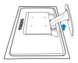
2. Press the locking clips to detach the base stand away from the base column.
