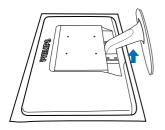
2. Hold the monitor base stand with both hands and firmly insert the base stand into the base column.
