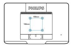
2. Remove the 4 screws and then remove the base from the monitor.
