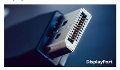
DisplayPort is a digital link from PC to monitor without any conversion. With higher capabilities than DVI standard, it is fully capable to support up to 15 metre cables and 10.8 Gbps/sec data transfer. With this high
