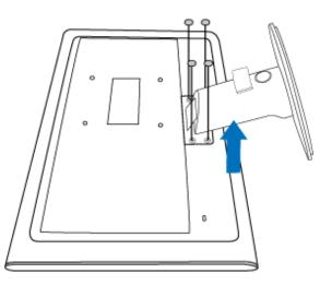
Remove the 4 screws and then remove the base from the LCD monitor.
