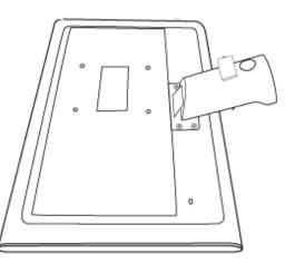
2) Hold the monitor base with both hands and firmly insert the base stand into the base column.
