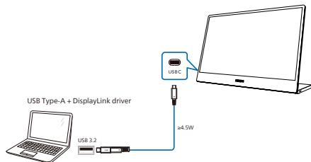
Note: Compatible with USB 3.2 on DisplayLink, not USB 2.0.
