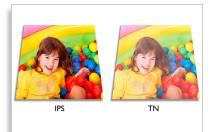
IPS displays uses an advanced technology which gives you extra wide viewing angles of 178/178 degree, making it possible to view the display from almost any angle - even in 90 degree Pivot mode! Unlike standard TN panels, IPS displays gives you remarkably crisp images with vivid colors, making it ideal not only for Photos, movies and web browsing, but also for professional applications which demand color accuracy and consistent brightness at all times.
