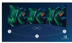
IPS displays use an advanced technology which gives you extra wide viewing angles of 178/178 degree, making it possible to view the display from almost any angle. Unlike standard TN panels, IPS displays gives you remarkably crisp images with vivid colors, making it ideal not only for Photos, movies and web browsing, but also for professional applications which demand color accuracy and consistent brightness at all times.
