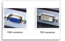
Dual input provides connectors to accommodate input of both analog VGA and digital DVI signals.
