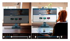
PowerSensor is a built-in 'people sensor' that transmits and receives harmless infrared signals to determine if user is present and automatically reduces monitor brightness when user steps away from the desk, cutting energy costs by up to 70 percent and prolonging monitor life.
