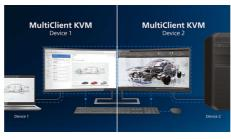
With MultiClient Integrated KVM switch, you can control two separate PCs with one monitor-keyboard-mouse set up. A convenient button allows you to quickly switch between sources. Handy with set-ups that require dual PC computing power or sharing one large monitor to show two different PCs.
