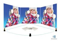
IPS-ADS displays use an advanced technology that gives you extra-wide viewing angles of 178/178 degrees, making it possible to view the display from almost any angle. Unlike standard TN panels, IPS-ADS displays give you remarkably crisp images with vivid colours, making them ideal not only for Photos, movies and web browsing, but also for professional applications that demand colour accuracy and consistent brightness at all times.
