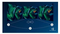
IPS displays use an advanced technology which gives you extra wide viewing angles of 178/178 degree, making it possible to view the display from almost any angle - even in 90 degree Pivot mode! Unlike standard TN panels, IPS displays gives you remarkably crisp images with vivid colors, making it ideal not only for Photos, movies and web browsing, but also for professional applications which demand color accuracy and consistent brightness at all times.
