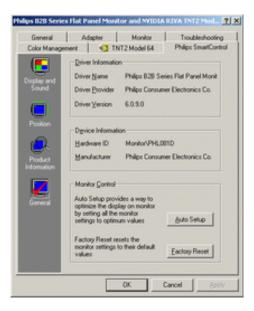
Within monitor control, users can click on Auto Setup to achieve optimum performance or click on factory reset to reset the parameters of the monitor. Such choices are disabled when using DVI-D (digit) input.
