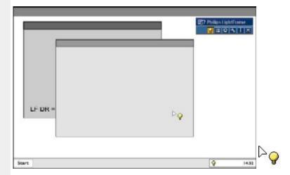
Your cursor becomes a yellow light bulb when it passes over a **non-active** window to indicate that LightFrame<sup>TM</sup> DR can be activated in the selected window. Click to activate LightFrame<sup>TM</sup> DR in the selected window. To activate LightFrame<sup>TM</sup> DR simultaneously in a total of up to eight windows, click on the selected windows one-by-one while pressing the *Shift* key.
