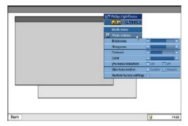
3. Change settings by pulling the color bar or pressing the plus (+) or minus (-) button to move incrementally to the desired levels.
