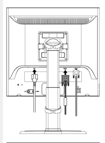
1) Plug in the cables into connectors.
