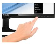
Touch controls are intelligent, touch-sensitive icons that replace protruding buttons so the user can adjust the monitor to their requirements. Responding to your lightest touch, touch controls give the monitor a modern feel.
