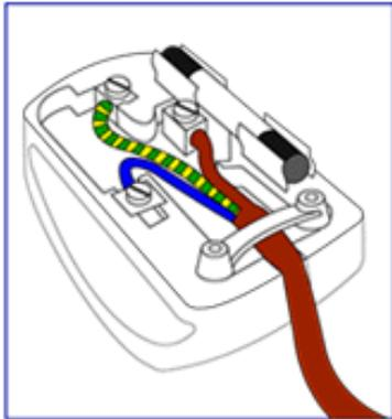
Before replacing the plug cover, make certain that the cord grip is clamped over the sheath of the lead - not simply over the three wires.
