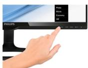
Touch controls are intelligent, touch sensitive icons that replace protruding buttons that lets the user adjust the monitor to their
