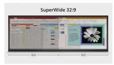
32:9 SuperWide 49" screen with 5120 x 1440 resolution is designed to replace multiscreen setups for a massive wide view. It's like having two 27" 16:9 Quad HD displays side by side. SuperWide monitors offer the screen area of dual monitors without the complicated setup.
