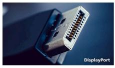
DisplayPort is a digital link from PC to monitor without any conversion. With higher capabilities than DVI standard, it is fully capable to support up to 15 metre cables and 10.8 Gbps/sec data transfer. With this high performance and zero
