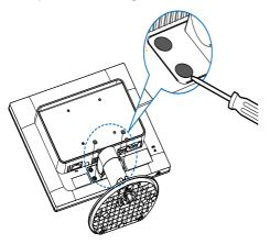
3. Remove the screws from hinge cover.
