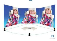
AH-IPS displays use an advanced technology which gives you extra wide viewing angles of 178/178 degree, making it possible to view the display from almost any angle. Unlike standard TN panels, AH-IPS displays gives you remarkably crisp images with vivid colors, making it ideal not only for Photos, movies and web browsing, but also for professional applications which demand color accuracy and consistent brightness at all times.
