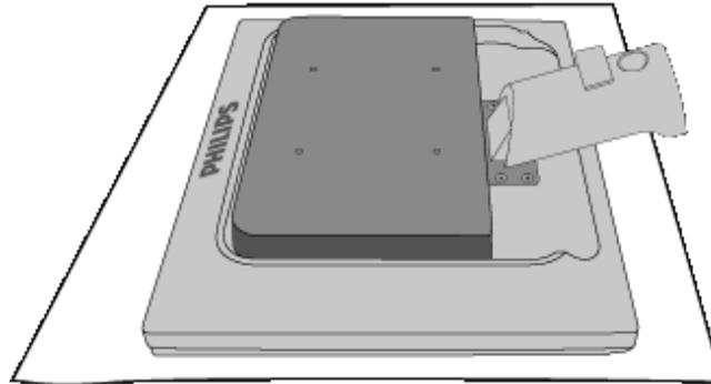
2) Hold the monitor base with both hands and firmly insert the base stand into the base column.
