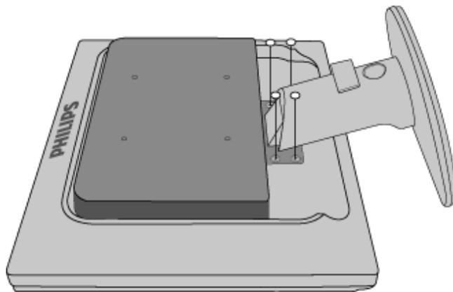
Remove the 4 screws and then remove the base from the LCD monitor.
