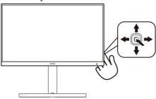
To access the OSD menu on this Philips display simply use the single toggle button on the rear side of the display. The single button operates like a joystick. To move the cursor, simply toggle the button in four directions. Press the button to select desired option.
