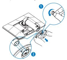
3. Remove the screws from hinge cover.
