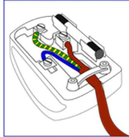
1. The GREEN AND YELLOW wire must be connected to the terminal in the plug which is marked with the letter "G" or by the Ground symbol  $\perp$  or coloured GREEN or GREEN AND YELLOW.
