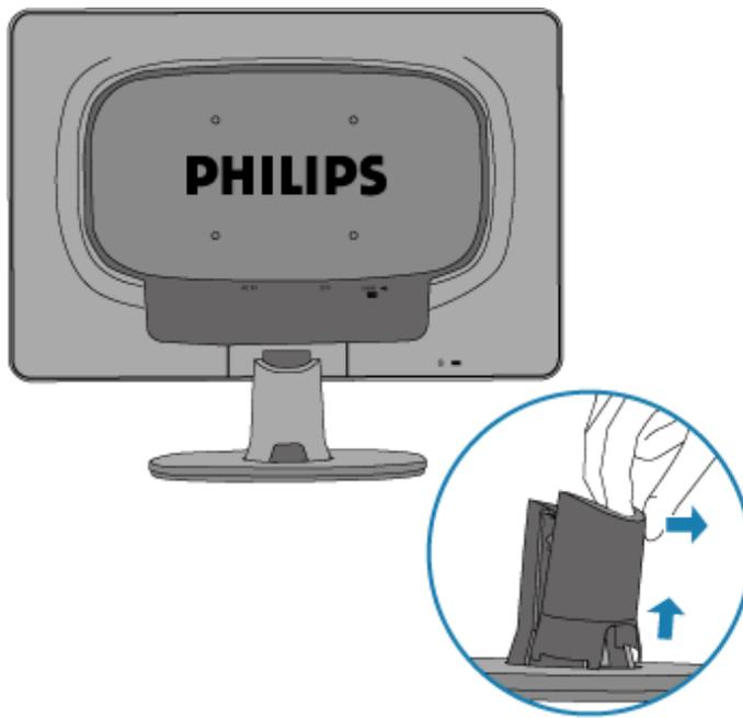
2) Place the monitor face on a safe surface, push down on the release button and pull the base away from the monitor body.
