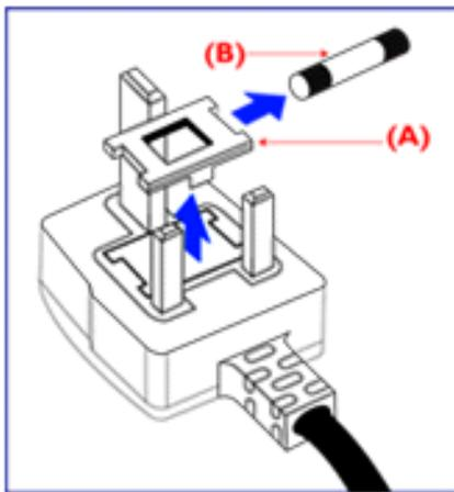
If the mains plug contains a fuse, this should have a value of 5A. If a plug without a fuse is used, the fuse at the distribution board should not be greater than 5A.
