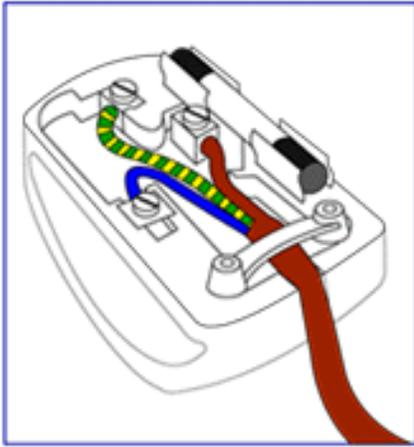
1. The GREEN AND YELLOW wire must be connected to the terminal in the plug which is marked with the letter "E" or by the Earth symbol
