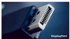
DisplayPort is a digital link from PC to monitor without any conversion. With higher capabilities than DVI standard, it is fully capable to support up to 15 metre cables and 10.8 Gbps/sec data transfer. With this high performance and zero latency, you get the fastest imaging and refresh rates — making DisplayPort the best choice for not only general office or home use, but also for
