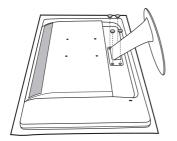
2. Remove the 4 screws and then remove the base from the monitor.
