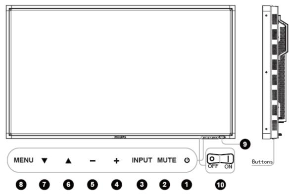
**OPOWER button** (()): To switch the power on/off.
