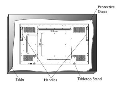
I. Lay a protective sheet on a table, which was wrapped around the monitor when it was packaged, beneath the screen surface so as not to scratch the screen face.
