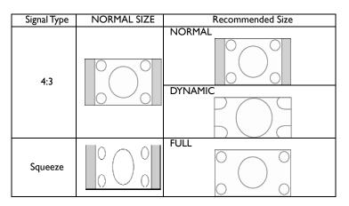
NORMAL: Display with the input signal aspect ratio from PC signal, or display in 4:3 aspect ratio at CVI or VIDEO signal.
