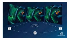
IPS displays use an advanced technology which gives you extra-wide viewing angles of 170/170 degrees, making it possible to view the display from almost any angle. Unlike standard TN panels, IPS displays gives you remarkably crisp images with vivid colours, making it ideal not only for Photos, movies and web browsing, but also for professional applications which demand colour accuracy and consistent brightness at all times.
