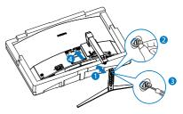
3. After attaching the base, erect the monitor with both hands on holding the monitor together with styrofoam firmly. Now you can pull out the styrofoam. When you pull out the styrofoam, do not squeeze the panel to avoid broken panel.
