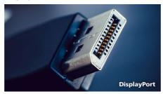
DisplayPort is a digital link from PC to Monitor without any conversion. With higher capabilities than DVI standard, it is fully capable to support
