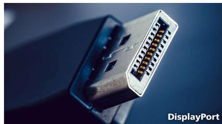
DisplayPort is a digital link from PC to monitor without any conversion. With higher capabilities than DVI standard, it is fully capable to support up to 15 metre cables and 10.8 Gbps/sec data transfer. With this high performance and zero latency, you get the fastest imaging and refresh rates — making DisplayPort the best choice for not only
