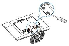
3. Remove the screws from hinge cover.
