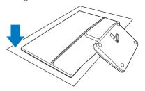
2. Hold the monitor and base with both hands. Gently bend the base vertically down to a fixed angle.
