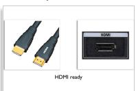
A HDMI-ready device has all the required hardware to accept High-Definition Multimedia Interface (HDMI) input, high quality digital video and audio signals all transmitted over a single cable from a PC or any number of AV sources including set-top boxes, DVD players and A/V receivers and video cameras.
