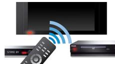
EasyLink uses the HDMI CEC industry standard protocol to share functionality between connected devices and the TV. With EasyLink only one remote control is needed to operate main functionalities on your TV and connected devices. EasyLink uses the standard HDMI cable to transfer system commands. It works between all electronic devices equipped with HDMI CEC.
