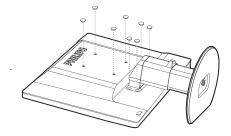
2. Remove the 4 screws and then remove the base from the monitor.
