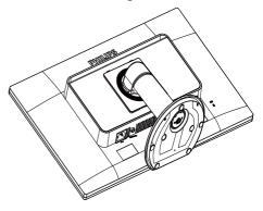
2. Remove the screws from hinge cover.
