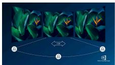
IPS displays use an advanced technology that gives you extra-wide viewing angles of 178/178 degrees, making it possible to view the display from almost any angle. Unlike standard TN panels, IPS displays give you remarkably crisp
