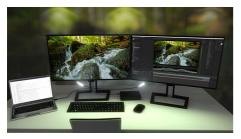
Daisy chaining allows you to drive multiple monitors and devices from a single Thunderbolt port on your laptop. From the Thunderbolt port of your laptop connect to this monitor, then from the second Thunderbolt port on this monitor you can connect to a second 4K monitor.
