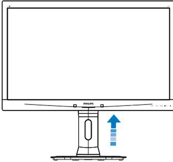
2. Place the monitor face down on a smooth surface. Pay attention not to scratch or damage the screen. Then lift the monitor stand.
