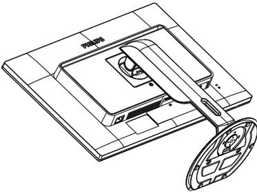
3. While keeping the release button pressed, tilt the base and slide it out.
