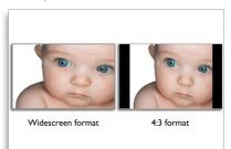
Philips auto picture format is a button that switches from the 4:3 aspect ratio to the widescreen mode, and back again, to match the display's aspect ratio with your content for working with wide documents without scrolling or viewing widescreen media in the widescreen mode and distortion-free, native mode display of 4:3 ratio content.
