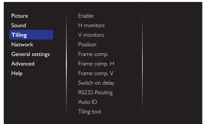
Create a single large-screen matrix (video wall) that consists of up to 100 sets of display (up to 10-sets on the vertical and 10-sets on the horizontal sides).
