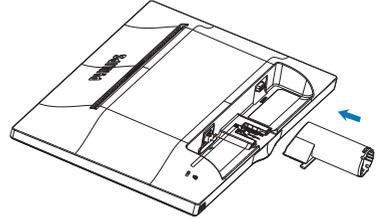
3. Hold the monitor base stand with both hands and firmly insert the base stand into the base column.
