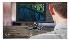
PowerSensor is a built-in 'people sensor' that transmits and receives harmless infrared signals to determine if user is present and automatically reduces monitor brightness when user steps away from the desk, cutting energy costs by up to 75 percent and prolonging monitor life.
