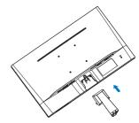
Hold the monitor base stand with both hands and firmly insert the base stand into the base column.
