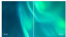
The 10-bit display delivers rich colour depth with 1.074 billion colours and 12-bit internal processing for recreating smooth, natural colours without gradations and colour banding.
