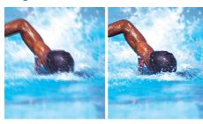
Progressive Scan doubles the vertical resolution of the image resulting in a noticeably sharper picture. Instead of sending a field comprising the odd lines to the screen first, followed by the field with the even lines, both fields are written at one time. A full image is created instantaneously, using the maximum
